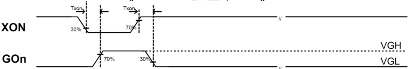
Figure 5.2.2 Gate driver input timing (continued)
